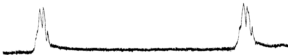
Fig. 3.—C-Methyl (left) and N-methyl (right) resonances of N-methylacetamide at very high resolution; pH about 13. The spin-spin interaction between the two methyl groups is about 0.45 c./s.
