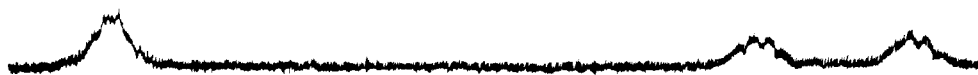
Fig. 4.—C-Methyl (left) and N-methyl (doublet at right) resonances of N-methylacetamide at very high resolution; pH about 5.
